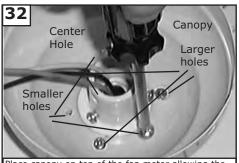
Place canopy on top of the fan motor allowing the yoke, wires and safety cable to pass through the large hole in the center of the canopy. Align the 3 larger holes around the center hole with the 3 screws still installed in the fan. Install 3 screws removed into small holes in canopy to make it a flush mount canopy and tighten screws securely.
